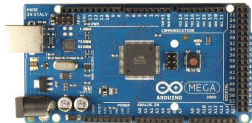
**Figure 9 – Arduino Mega 2560**
