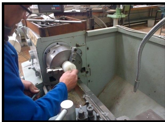
Figure 9: Lathing of flow meter flanges in EEW
