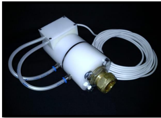
Figure 10: Assembled custom orifice flow meter
